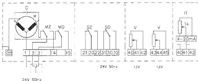
Stellsignal 0-10 V, 0(4)-20 mA, Versorg.-spann. 24 V/50 Hz
