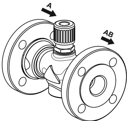
$t_{max} = 150^{\circ}\text{C}; \text{PN } 16$
