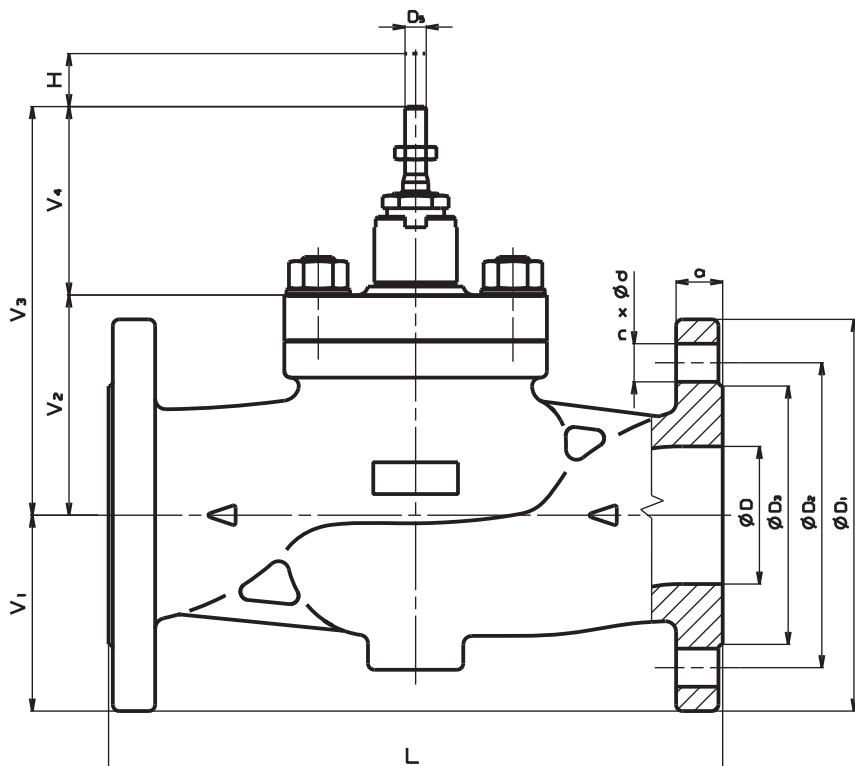
**Dimensions and weights of valves made of spheroidal cast iron for the type
