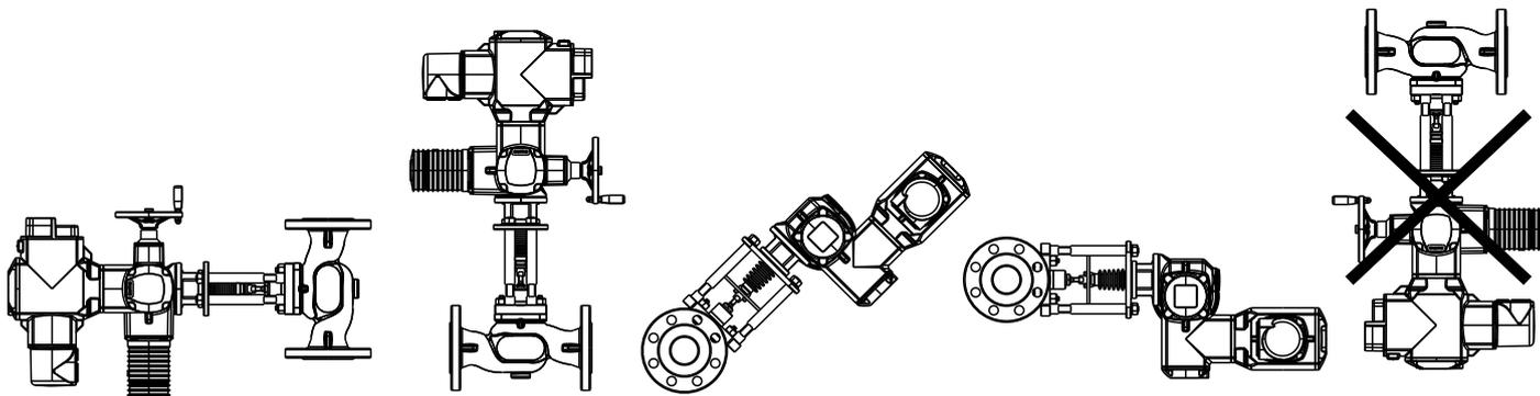
Pic. 3: Installation position for valves with electro actuators
