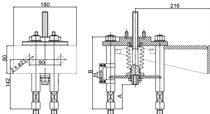
Pic.4: Fixing bracket for DN15 to 25 valves.
