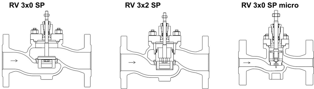
Pic.1: Flow direction for two-way valve with V-ported or contour plug
