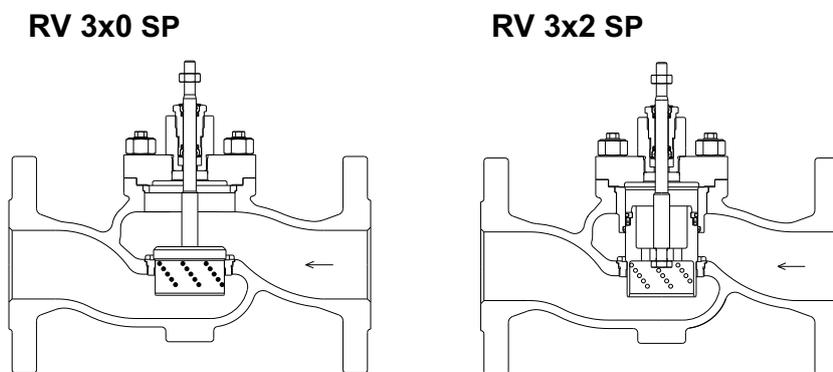
Pic.2: Flow direction for valve with perforated plug
