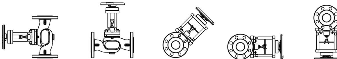
Pic. 5: Installation position for valves with hand wheel
