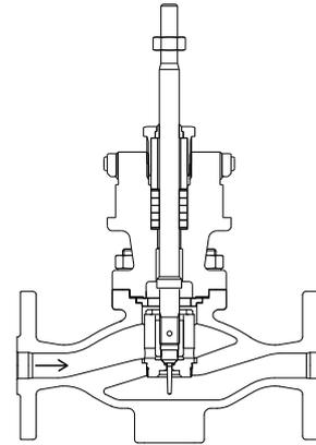
Pic.1: Flow direction for two-way valve with V-ported or contour plug
