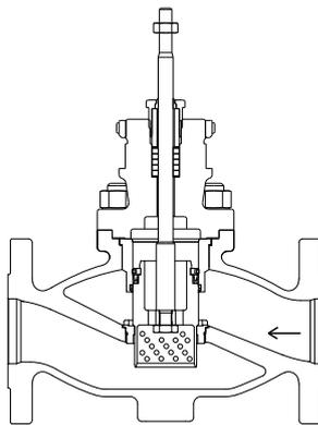
Pic.2: Flow direction for valve with perforated plug
