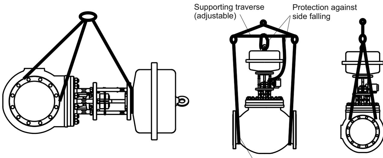
Pic. 8: Example of lifting device usage.
